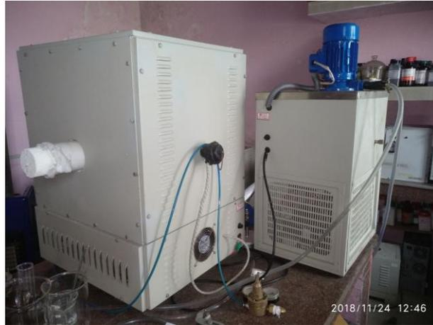
Fig.1 High temperature tube furnace with controlled Ar and N<sub>2</sub> gas purging.
