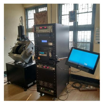
Fig.1 MicroSense (USA) 2.7 Tesla VSM
