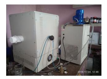
Fig.1 High temperature tube furnace with controlled Ar and N2 gas purging.
